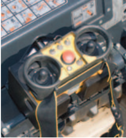
Removable operating console with standard dual function cabled / radio remote control. This control allows walk behind as well as remote operation.
