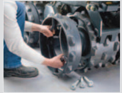
Easy installation of standard bolt-on drum extension increases compactor versatility.
